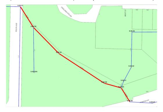
The Sewer pipe segments that make up the work are shown below:
